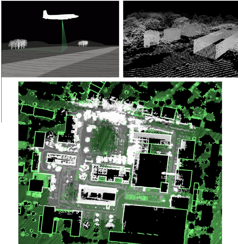
Fig. 7. Top left: Schema of the airborne based acquisition of reference data. Top right: 3D map consisting of aerial laser data and extrapolated 2D reference data. Bottom: Airborne and 3D map (black) with superimposed 3D scans (gray).
