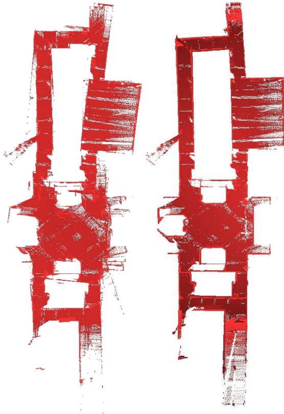
Figure 2. Top view of 3D laser scans before (left) and after correction (right) with 900 iterations of LUM. The data results from 64 scans each containing 81225 ( 225 \times 361 ) data points.
