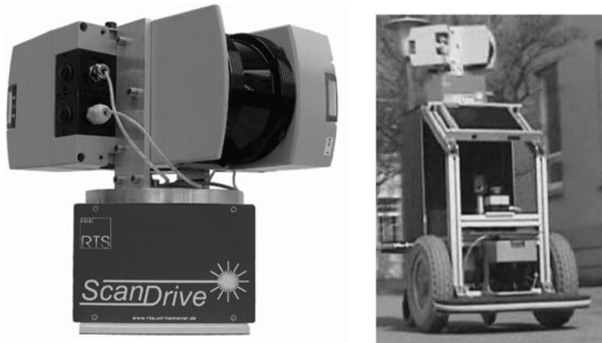
Figure 2. Left: 3D laser range sensor RTS/ScanDriveDuo. It takes a full 3D scan of 32,580 points in 1.2 s. Right: The mobile robot Erika.
